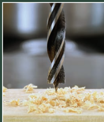
Brad Point (or Spur Point) Self-centering; wider spiral flutes clear waste easily. Produces ultra-clean holes in wood. Sizes: 5/64" to 1"; 1/8" to 1/2" most common.
