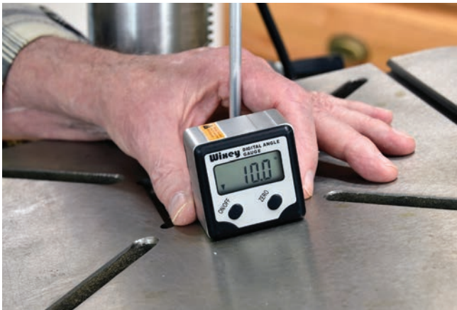
Once zeroed to the table, a digital angle gauge gives an exact reading as the table is rotated into position for angled drilling. One of these handy gauges will earn its keep with all sorts of tool setups.
