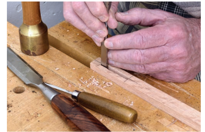
To complete the mortise, use chisels to remove the remaining waste left over from the drilling process, and square up the mortise ends if desired.
