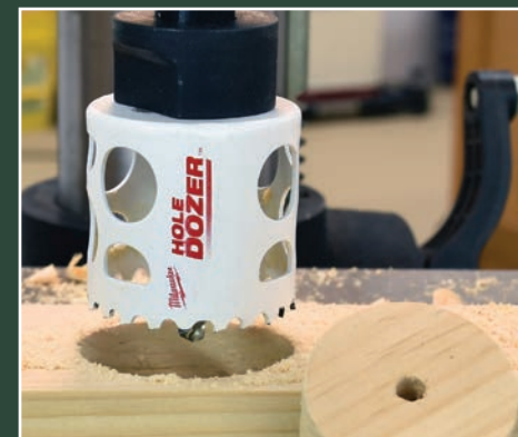
Hole Saw Multi-material use; excellent for larger holes in sheet stock or drywall. Central pilot bit keeps saw cutting around a single axis. Does not produce the cleanest holes. Sizes: 5/8" to 6".
