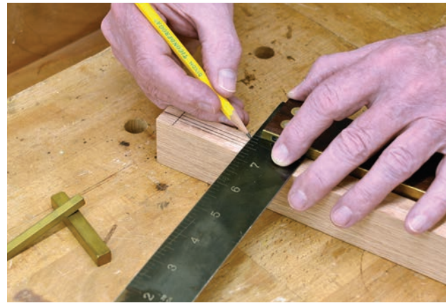
The most important details of laying out a mortise for drill press cutting is a center line and stop lines on the workpiece. Drill only inside the lines.
