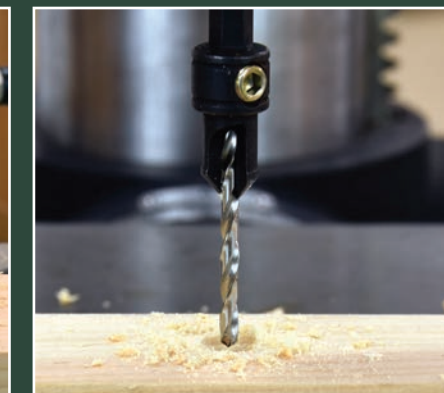
Countersink Bit Variations with or without pilot bit, creates countersink or counter bore to lower screwheads below the material surface. Sizes: Typically correspond to common screw/bolt heads.
