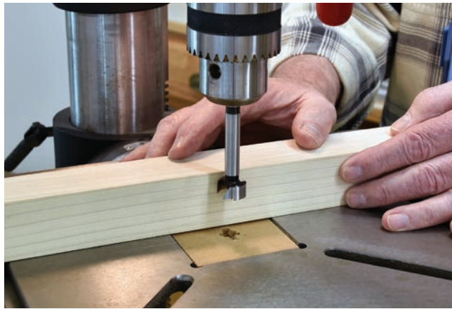
For cutting mortises, use a Forstner bit matching the workpiece thickness to set and lock the fence. Then, swap the Forstner bit for your drill bit, and the mortise you drill will be perfectly centered.
