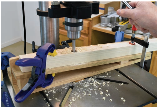
If you build numerous projects needing the same angled holes, making a jig for the task eliminates the need for tilting the table – it always stays at its original 90 degrees.
