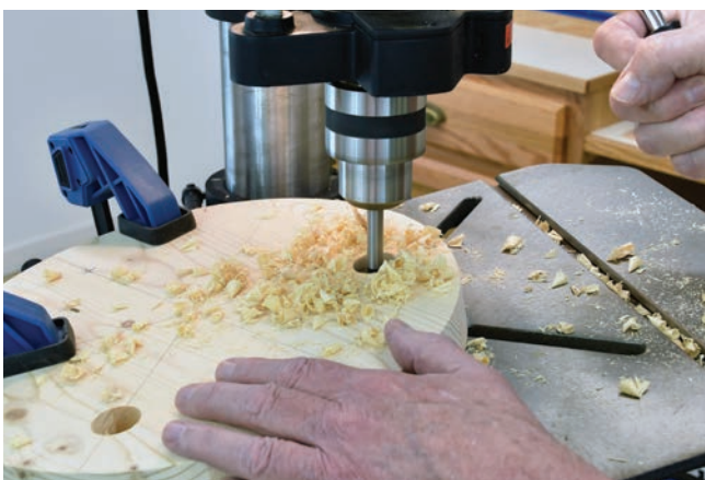
With workpiece drilling locations marked, clamp the stock in place and set the depth stop. Then just drill, rotate, reclamp and repeat.
