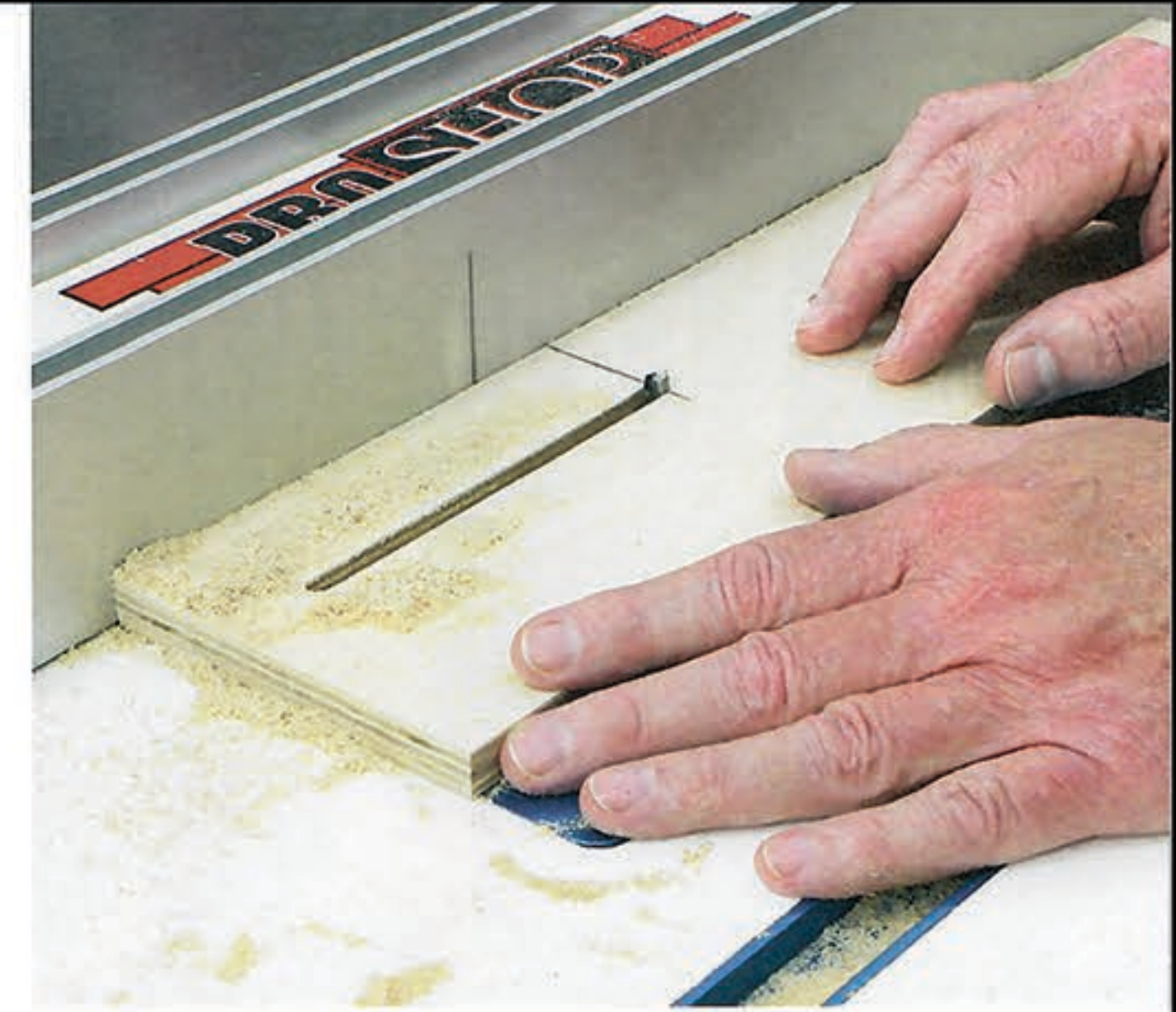
To make a routed slot inside a workpiece, line it up with your start mark on the fence. Then just drop, rout to your stop mark and lift up. The location of the slots may need to be adjusted to accommodate your drill press.
