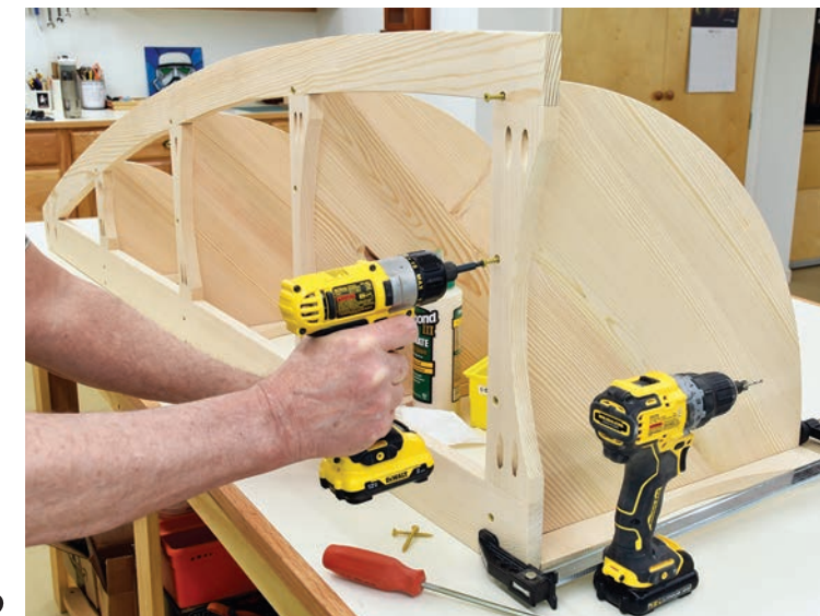
Apply waterproof glue to the shelf edges and clamp them into place, then drive exterior screws in from the back to secure the shelves.
