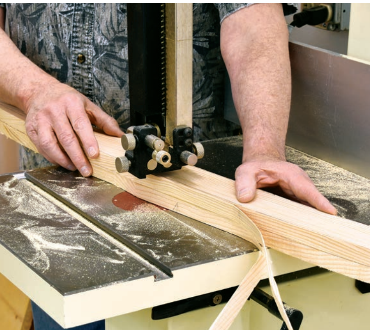
With the workpieces doubled up and pin-nailed together, cut both curved uprights at the same time. Once separated, the two components will be mirror-imaged and a perfect match.
