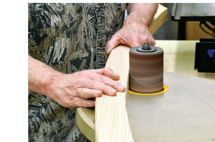
A spindle sander makes fast work of refining the concave sides of the doubled curved uprights, while a disc sander handles the convex sides.
