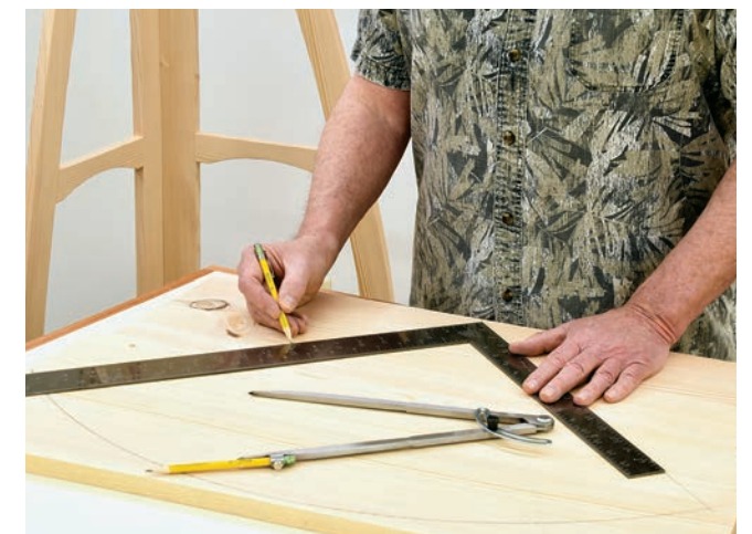
Use a compass or trammel to draw the arc for each shelf, then follow up with a carpenter's square to mark its two flat edges. Pivot the square to avoid knots and flaws on shelf edges, if needed.
