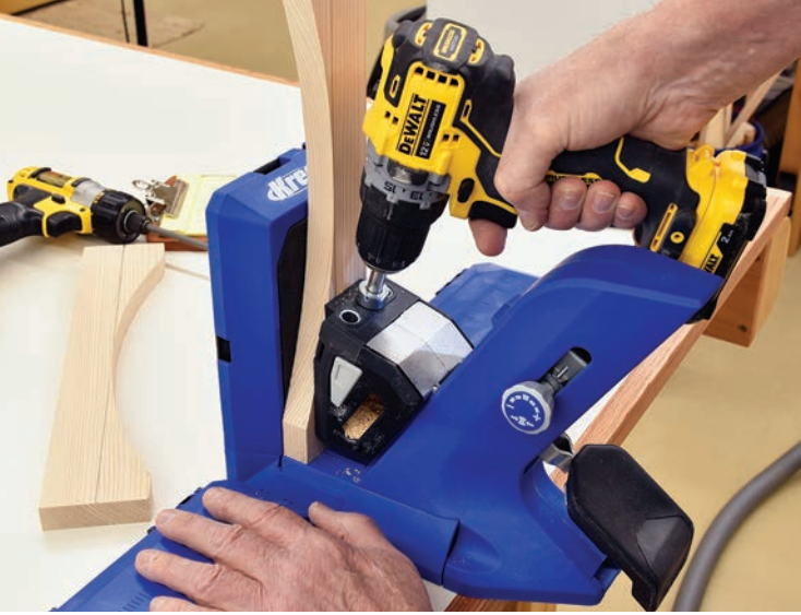
Pocket holes are the fastest and easiest method of joinery for the rails in each of the side frames. Orient the screws so they're unseen on the backs of the components.
