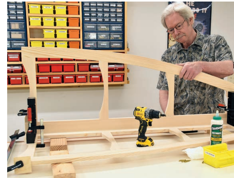
With both side frames complete, add a bit of exterior glue to the rabbets along the back edges, and screw the two halves together at 90 degrees.
