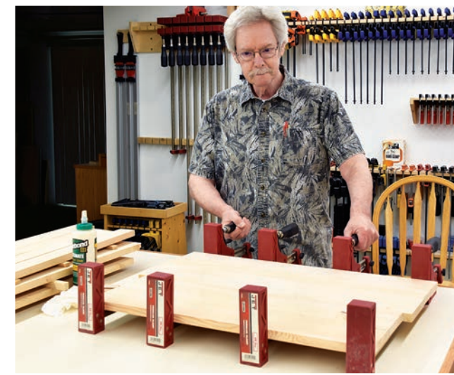
Glue up panels for the four shelves from narrower boards. It's good practice to alternate growth rings in these instances, especially if your stock is wide, to help minimize warping. Be sure to use waterproof glue for these assemblies.
