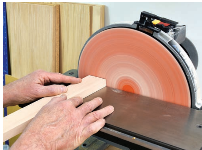
Round one end of each rail to your layout lines so they'll fit against the inner edge of the curved uprights. Sand carefully — you'll only need to remove a small amount of material to achieve the correct curve.
