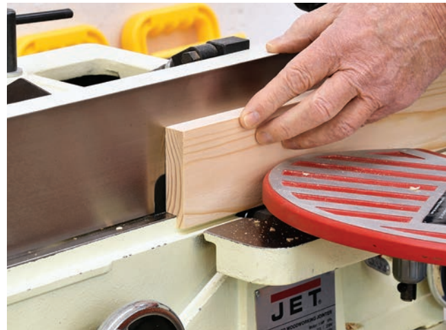
Use a dado blade on your table saw, a straight bit in a router table or, as the author is doing here, a jointer to create a 3/8" x 3/8" rabbet on the back edges of the straight rear uprights.
