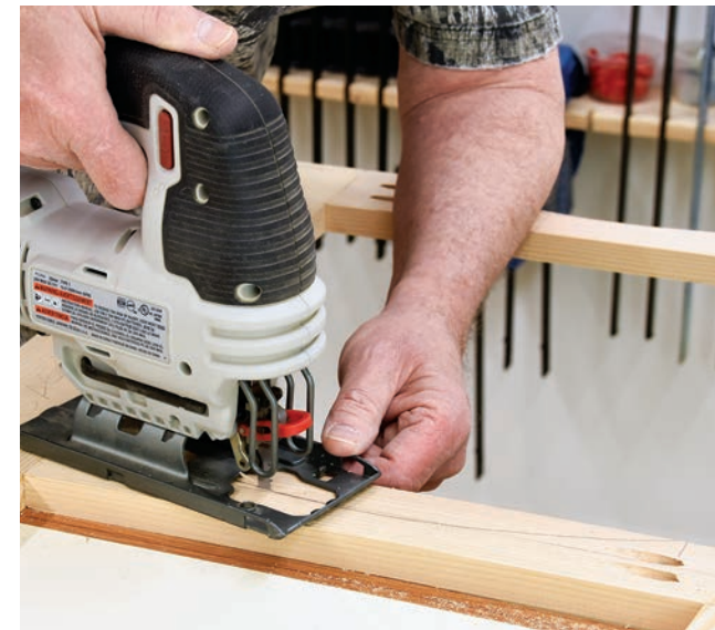
The decorative curves under each rail can be cut on a band saw before assembly, but lacking a band saw it's easier to install the rails first and then jigsaw the curves.
