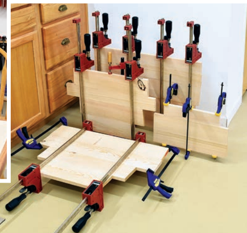
Glue up panels for the four shelves from narrower boards. It's good practice to alternate growth rings in these instances, especially if your stock is wide, to help minimize warping. Be sure to use waterproof glue for these assemblies.
