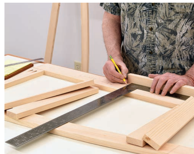
With the side frames pocket-screwed together at the top and bottom, measure the rail locations to get the exact lengths needed. Don't forget to account for the curve on one end of each rail.
