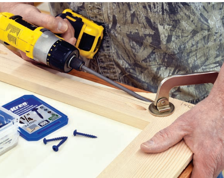
Begin assembly of the side frames by applying a bit of glue to the ends of the bottom rails, then drive in the pocket screws. Once again, use an exterior-rated glue.
