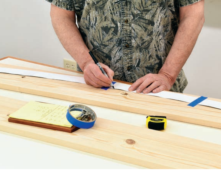
Transfer the pattern for the curved uprights to the stock, taking care to avoid knots in these narrow components. Masking tape can help keep the pattern from moving around as you trace.
