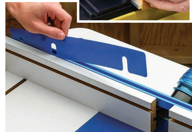
Commercial router fences usually offer easy ways to shim the left sub-fence for jointing. Typical methods include slip-in shims that go behind the sub-fence or insertable bars that slide in from the end.
