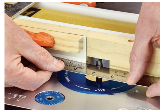
With the laminate clamped to the face of the left portion of the sub-fence, use a straightedge to line up the bit with the laminate face. With a conventional straight bit, make sure the cutter is at the apex of its cutting path.
