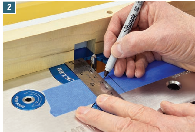
2 With the fence set, use a marker to establish the cutting edges of the router bit. The lines represent the forward and rear cutting edges.
