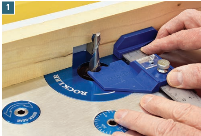
1 Set the fence distance to establish where the mortise will be cut in the workpiece. Rockler's router bit center/depth gauge makes this precise.
