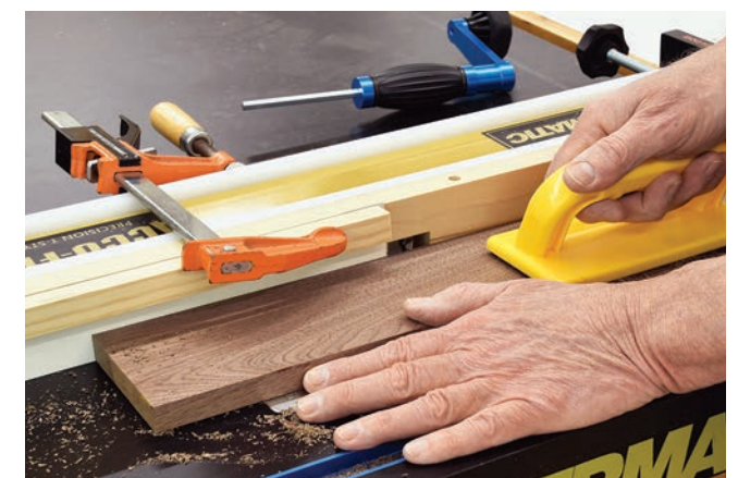
With the exception that the workpiece is flat on its face and the cutter is alongside it rather than underneath, the actual edge-jointing process is identical on a router table to that of a dedicated stationary jointer.
