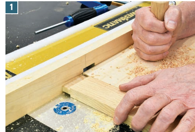
1 To make the tenon, set the bit to the desired height and create the tenon's faces in two passes over the bit. A backing board adds stability and safety.
