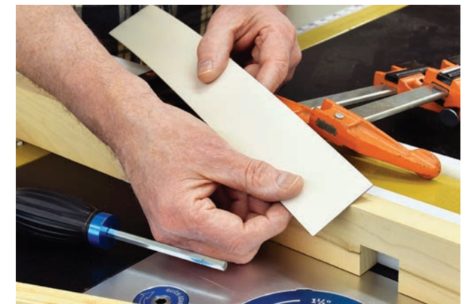
A narrow strip of general-purpose plastic laminate, about 1/16" thick, makes a perfect shim to offset a shop-made router table sub-fence on the left side of the bit for jointing.
