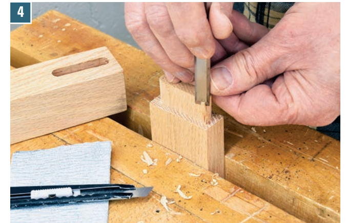
4 To fit the tenon properly into the mortise, the author opts to round off the tenon with a chisel and knife. Alternatively, you can square the ends of the mortise with a narrow chisel.
