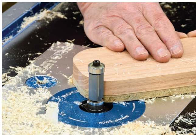
To keep the remainder of the cuts with the grain, flip the workpiece and raise the bit to expose the bit's bottom bearing. (Or switch to a bottom-bearing pattern bit instead.) Once adjusted, finish the routing pass.
