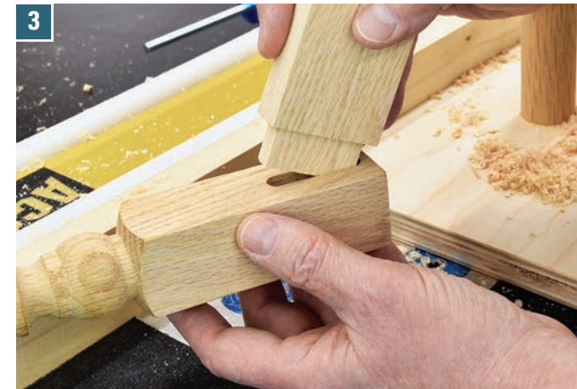
3 A test fit shows that all is good. The round mortise won't accept the squared tenon, of course, but we'll fix that in the next step.
