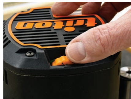
For tasks like jointing, you just don't need the full 20,000+ RPM of most routers. Dialing back the speed cuts noise and reduces potential burn marks on the wood.
