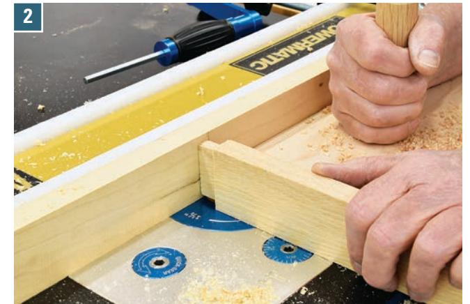
2 Turn create the tenon edge shoulders, repeat the process with the workpiece on its edge.
