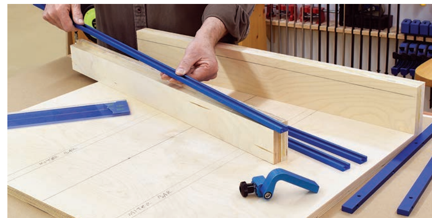
With all the major components and pieces cut, test fit everything before making shaping cuts and starting assembly. Here, the author has laid out locations for the central kerf and miter bars on the sled's base piece. He's also used the rear fence workpiece to mark its height on the front fence.
