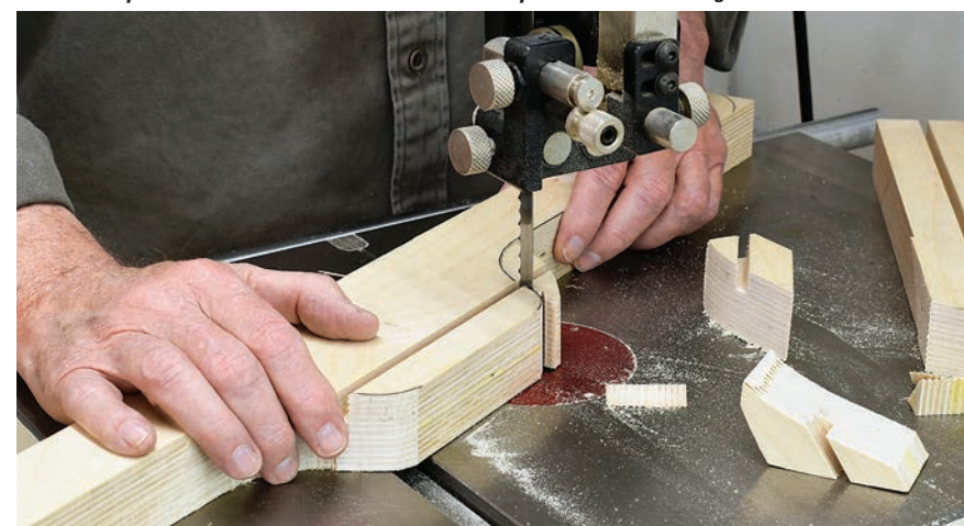
Cut the front fence to shape on the band saw. You may need to make relief cuts on sharper curves.
