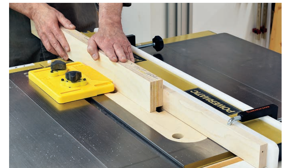
With a dado stack installed in the table saw, cut a 3/4" wide by 3/8" deep rabbet on the top edge of the rear fence to accept a T-track for a flip stop.
