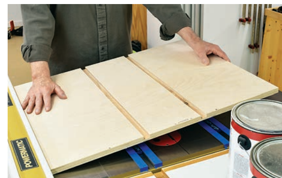
With the miter bars in place and a line of epoxy spread along their tops, register the sled base against the rip fence and carefully lower it onto the bars. Those paint cans shown here will weigh the plywood down until the glue cures.
