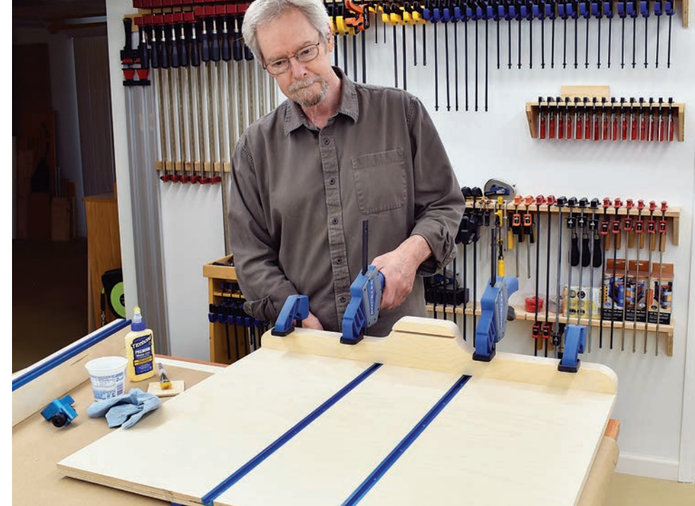
Glue and clamp the front fence into place on the front of the sled. When the glue dries, drive a couple of countersunk screws up from underneath to further reinforce this joint.
