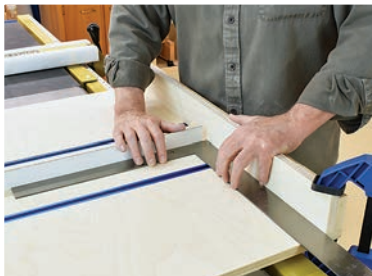
Place the sled on the saw and establish the main center kerf (above), but don't cut all the way through the back of the base yet. Note the piece of tape indicating a good stopping spot. A piece of hardboard in the kerf teamed with a reliable square help set the rear fence just right (inset). A screw on one end allows adjustment before clamping the fence down on the other end.
