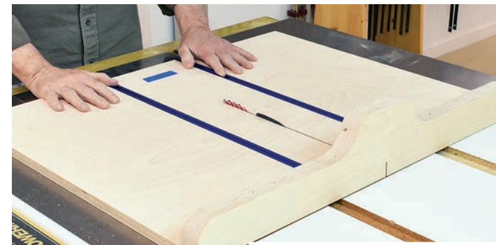
Place the sled on the saw and establish the main center kerf (above), but don't cut all the way through the back of the base yet. Note the piece of tape indicating a good stopping spot. A piece of hardboard in the kerf teamed with a reliable square help set the rear fence just right (inset). A screw on one end allows adjustment before clamping the fence down on the other end.
