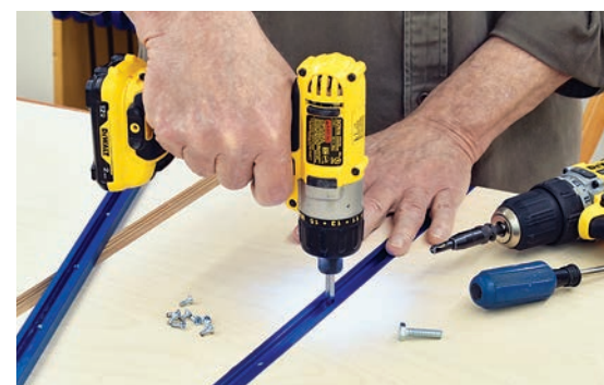
Use a self-centering bit to perfectly locate pilot holes, then securely attach the T-tracks into their dadoes in the top surface of the sled base.
