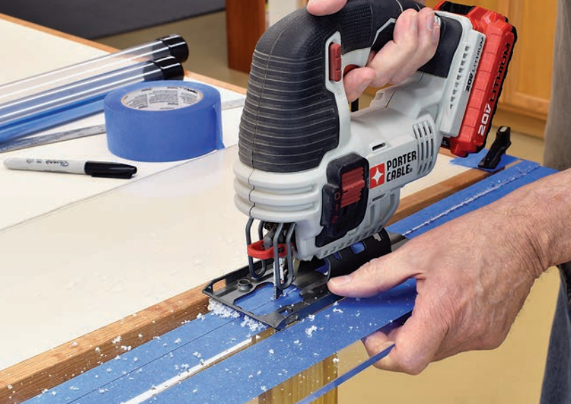
When cutting acrylic with a jigsaw, use a fine-tooth blade and set the orbital action as low as possible. Cut slowly to avoid overheating the plastic. A jointer set for a shallow cut makes quick work refining and smoothing the edges of acrylic (inset). Note the blue painter's tape used to keep from scratching the plastic.
