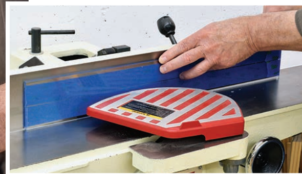
When cutting acrylic with a jigsaw, use a fine-tooth blade and set the orbital action as low as possible. Cut slowly to avoid overheating the plastic. A jointer set for a shallow cut makes quick work refining and smoothing the edges of acrylic (inset). Note the blue painter's tape used to keep from scratching the plastic.
