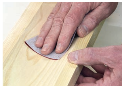
Once the cove is complete, sand off any "spiral" marks left by the saw blade.
