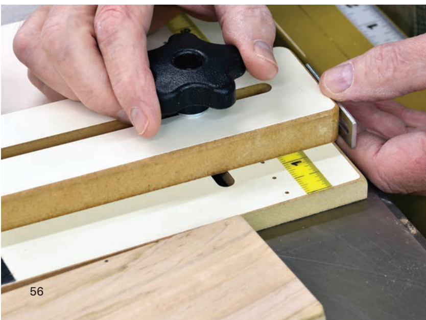
A rabbet cut made along the edge of a workpiece can be accomplished with the rip fence. Clamping on a sacrificial wooden fence protects the saw's regular fence facing.
