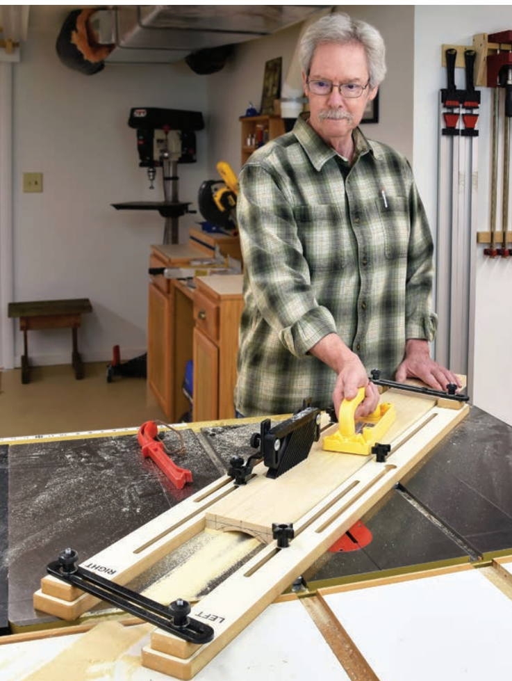
With the jig secured and featherboard in place, slowly feed the workpiece through the spinning blade, set initially at about 1/16" above the table. Raise the blade in small increments and make repeated cuts.
