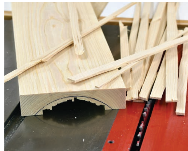
Coves create boatloads of dust. To minimize dust (and shorten cutting time), remove excess material before cutting the actual cove. Here, the author has made a series of straight rips and simply snapped out the waste.
