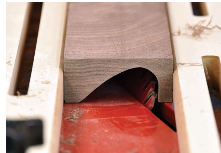
By tilting the saw blade, you can make coves in a variety of shapes. Here, the author is cutting walnut handles for a box project. After the cove is complete, individual handles are cut from the longer workpiece.
