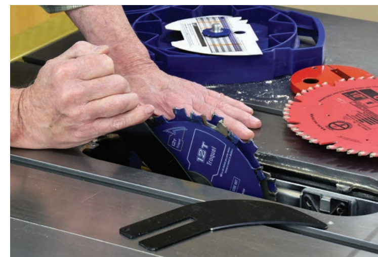
With blades, chippers and spacers "stacked," the set is secured in the table saw. Because dado sets are smaller than standard 10" blades, the riving knife must be removed. It serves no purpose for non-through cuts.
