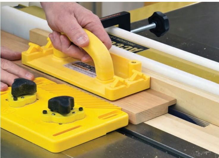
A rabbet cut made along the edge of a workpiece can be accomplished with the rip fence. Clamping on a sacrificial wooden fence protects the saw's regular fence facing.
