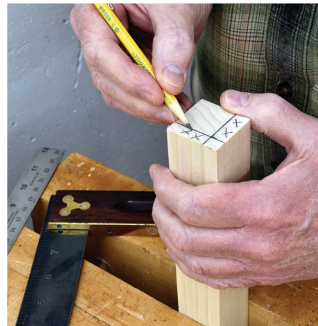
For this table leg, which will be tapered on two sides, the author pencils in the cutlines on the "foot" end of the leg showing where the tapering ends. There are also corresponding pencil marks at the beginning of the taper, higher up the leg.
