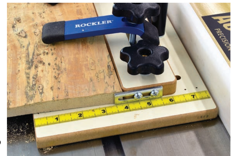
An adjustable stop at the rear of the jig works in tandem with the hold-down clamps to secure a workpiece during the cut.
