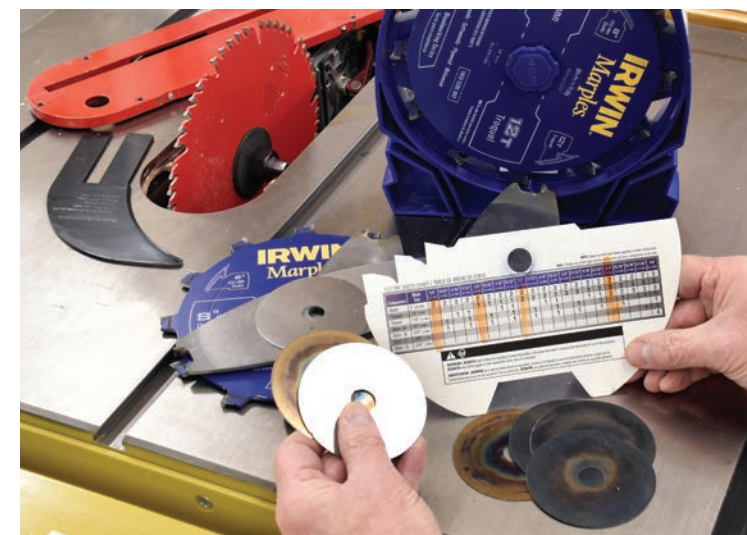
Standard dado sets include a pair of outer blades, a number of chipper blades and a series of shims and spacers to set and adjust dado widths. An included guide lists the parts needed for specific cuts.
