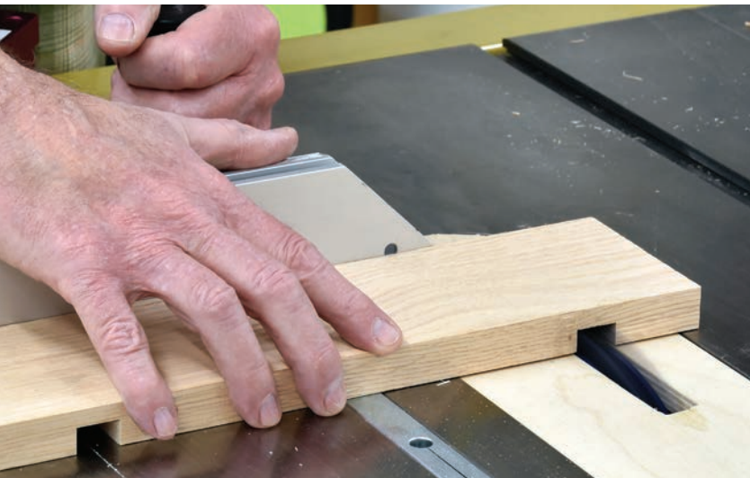
Non-through cuts like these dados are typically made using a miter gauge for narrow pieces and the saw fence for wider stock. Note that a custom throatplate sized for this specific dado setup creates a zero-clearance insert.
