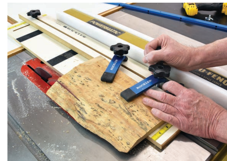
With the miter bar removed, the Rockler tapering jig works with the saw's rip fence as a straight-line jig to cut irregularly shaped workpieces. It's a safer way to get a straight edge.
