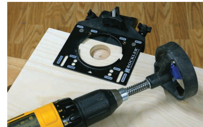
A cabinet door drilling jig paired with a 35 mm Forstner bit makes quick work of boring the mounting cup holes for Euro-style hinges.
