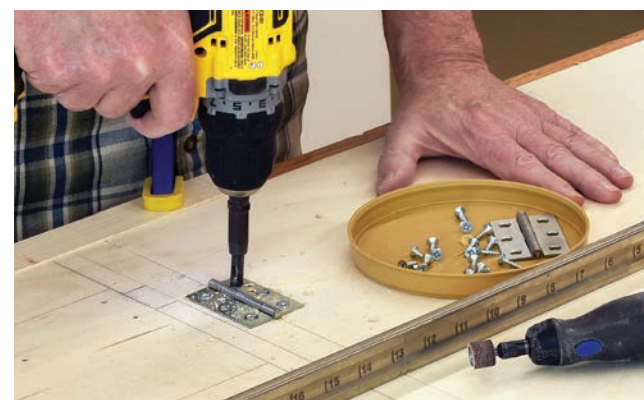
Before installing the main top to the cabinet assembly, mark, drill and attach the hinges and leaf supports temporarily to thread all pilot holes. You'll install the hardware permanently later in the building stage.
