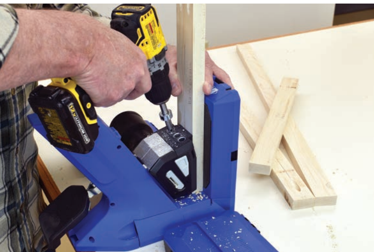
Drill pocket-screw holes in the solid-wood face frame rails, then assemble the frame on a flat surface with 1/4" pocket screws.
