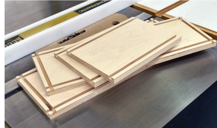
The author mills dados and rabbets first, then cuts the workpieces to final width when making particularly narrow parts. It's safer and more efficient.
