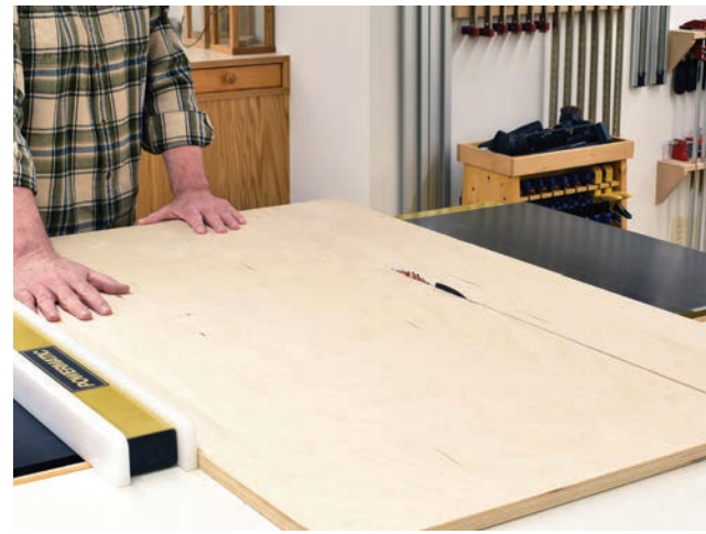
Cut all the plywood components at the table saw (or with a guided circular saw). During this process, orient workpieces so the blade cuts down into the face side of the stock for the cleanest cut.
