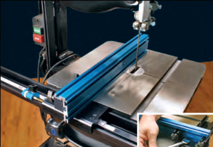
Any rip fence can guide stock; find one that's adjustable to compensate for drift. The Kreg fence adjusts to tweak the fence angle for a true feed.
