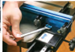
Any rip fence can guide stock; find one that's adjustable to compensate for drift. The Kreg fence adjusts to tweak the fence angle for a true feed.
