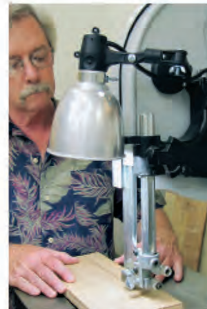
Even in well-lighted shops, cast shadows can make it difficult to follow cutting lines. A magnetic task light easily solves this problem.
