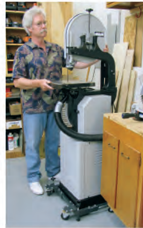
When space is an issue, a mobile base like the Shop Fox model shown here makes altering your shop layout a breeze.
