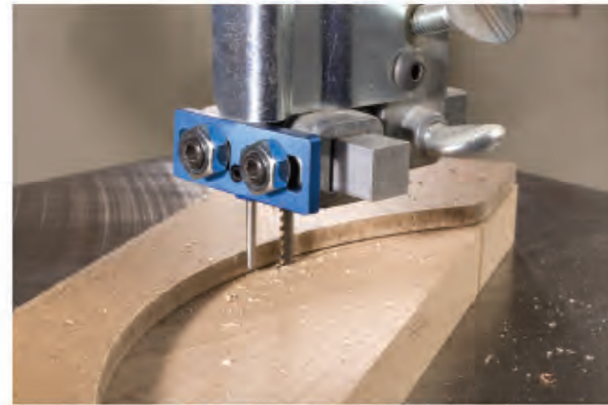
The Rockler duplicating pin allows fast and accurate template cutting on your hand saw — a process that not everyone associates with the band saw, but one that is quite handy.
